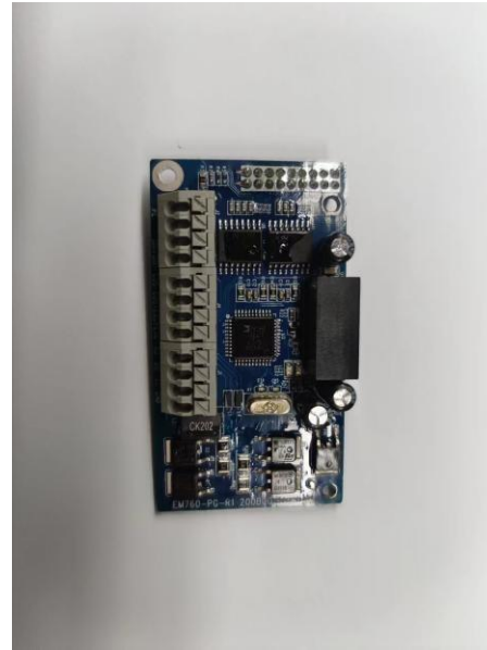
Fig. 9-20 Rotary transformer PG card - real product
