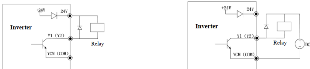
a: Use of internal power supply
